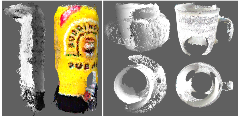
Figure 12: Shown here are a can and a mug aligned with ICP alone on the left of each image and our algorithm on the right. Due to the high level of symmetry in these objects, ICP is unable to find the correct alignments between sensor frames, resulting in largely useless object models.
