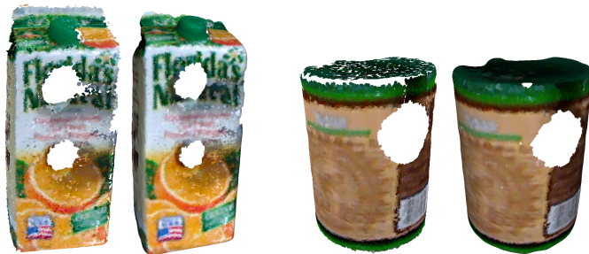
Figure 15: Surfel models and their respective meshed versions. Meshing can fill in small gaps between surfels such as the rim of the coffee can that was partially occluded by the palm. On the other hand, it struggles with thin surfaces like the top of the orange juice box and can smooth out sharp corners.
