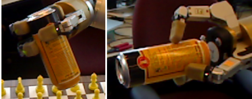
Figure 6: Two grasps of the same object. With just a single grasp, the resulting object model has holes. Any given part of the object is visible in at least one of the grasps.
