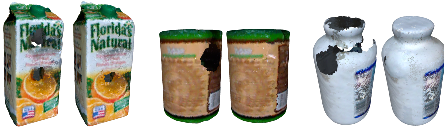
Figure 17: Side-by-side comparisons showing object models before and after regrasping. From left to right: an orange juice bottle, a coffee can, and a pill bottle. The regrasping procedure allows for holes caused by the manipulator to be filled in. In the case of the orange juice bottle, a small hole remains as there was some overlap between the grasp locations.
