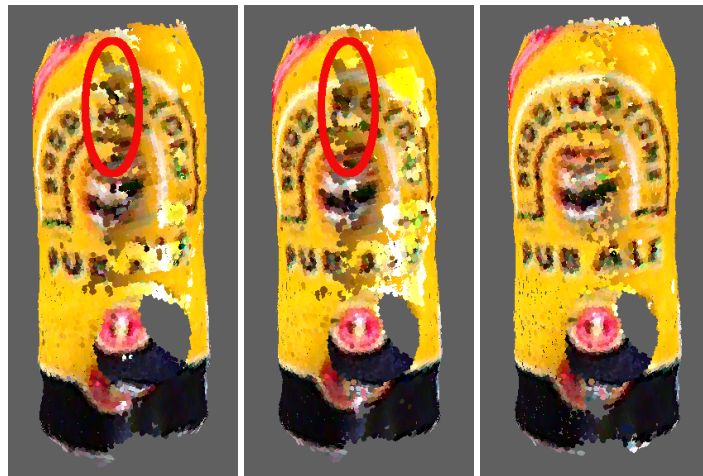
Figure 13: (left) Pre-loop closure can model without use of the dense color error term, (middle) with color error term, (right) with color error term after loop closure and surface merging.
