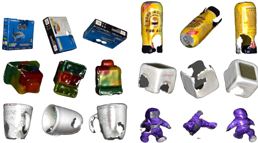
Figure 16: Triangulated surface models constructed from surfel clouds. Left column: a router box, large Lego pieces, and a mug. Right column: a can, a clock, and a stuffed doll. Holes in the models are due to occlusion by the hand or unseen regions due to the trajectory.
