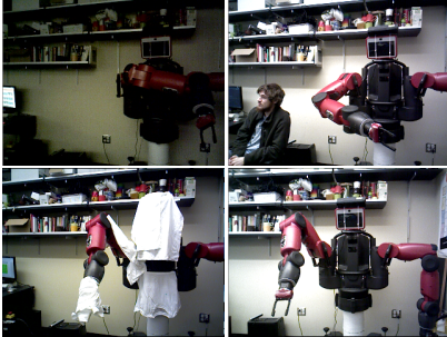
Fig. 5: Examples of different generalization tests. Clockwise from top left: 1) Low light setting, 2) Motion in the background (person on the chair), 3) Fixed distractor(s) in the foreground and 4) Change in camera pose (rotated \sim 10 degrees to the right).
