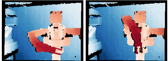
Fig. 1: An example scenario showing the initial (left) and target depth clouds (right). SE3-POSE-NETS can be used to control the robot to reach the target state based on raw depth (and optionally, color) data. Depth images colorized for display purposes only.
