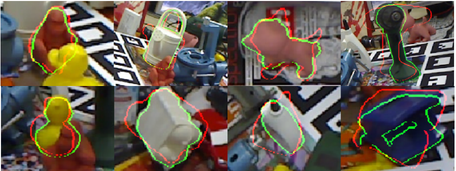
Fig. 6: Examples of refined poses on the Occlusion LILNEMOD dataset using the results from PoseCNN [29] as initial poses. The red and green lines represent the silhouettes of the initial estimates and our refined poses, respectively.
