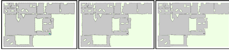
Fig. 6. Maps built during three autonomous exploration runs. The maps look almost identical, even though they were built under very different circumstances; (left to right) by one robot, by two robots starting from the same location, and by two robots starting from different, unknown locations. The similarity between the maps illustrates the robustness of the system and supports our belief that these maps are more accurate than the hand-built map.
