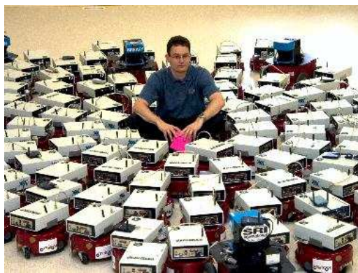
Fig. 1. 100 robots. Four of the robots are Pioneer IIs with SICK laser range-finders. The rest are Amigo-bots with sonars, a camera and a small PC on top. The OOI is in the hand of one of the authors.
