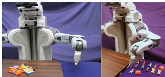
Fig. 1. One useful interaction with piles is the singulation of individual items. Interactive singulation enables a robot to perform tasks such as counting, arranging, or sorting of previously un-encountered objects.
