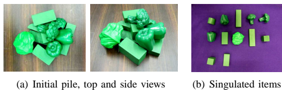
Fig. 9. For items without strong features, shape-based matching generates candidate rigid transforms. (a) Initial pile with several completely green items. (b) Singulated green items after interaction.
