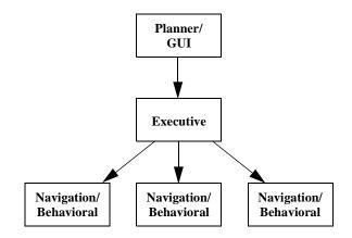
Figure 1: Tiered Architecture for Autonomous Robots
