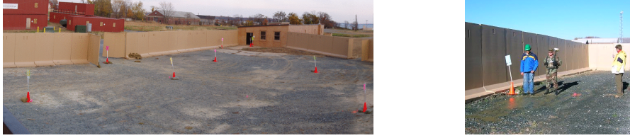
Fig. 3. Experimental setup: (left) Part of the evaluation area with waypoints. The subjects followed fully scripted traversals through the area. (right) A soldier and one of our team members wore a sensor system. Ground truth annotations were provided by four additional observers equipped with stop watches and audio recorders.
