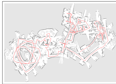
Fig. 11. Map created with the standard Rao-Blackwellized particle filtering technique in real-time using 100 samples and based on the raw odometry data.
